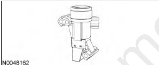
Typical IFS Switch
